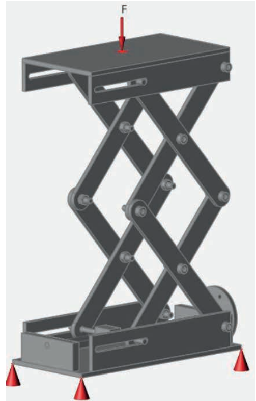
Figure 10 – Model made in finite elements showing loads and constraints
