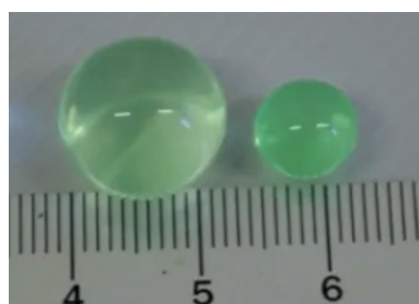
Figure 3. The hydrogel beads were calibrated with 0 M and 2 M NaCl.
