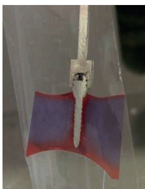
Fig. 2: Specimen after cutting in the Exakt® machine.
